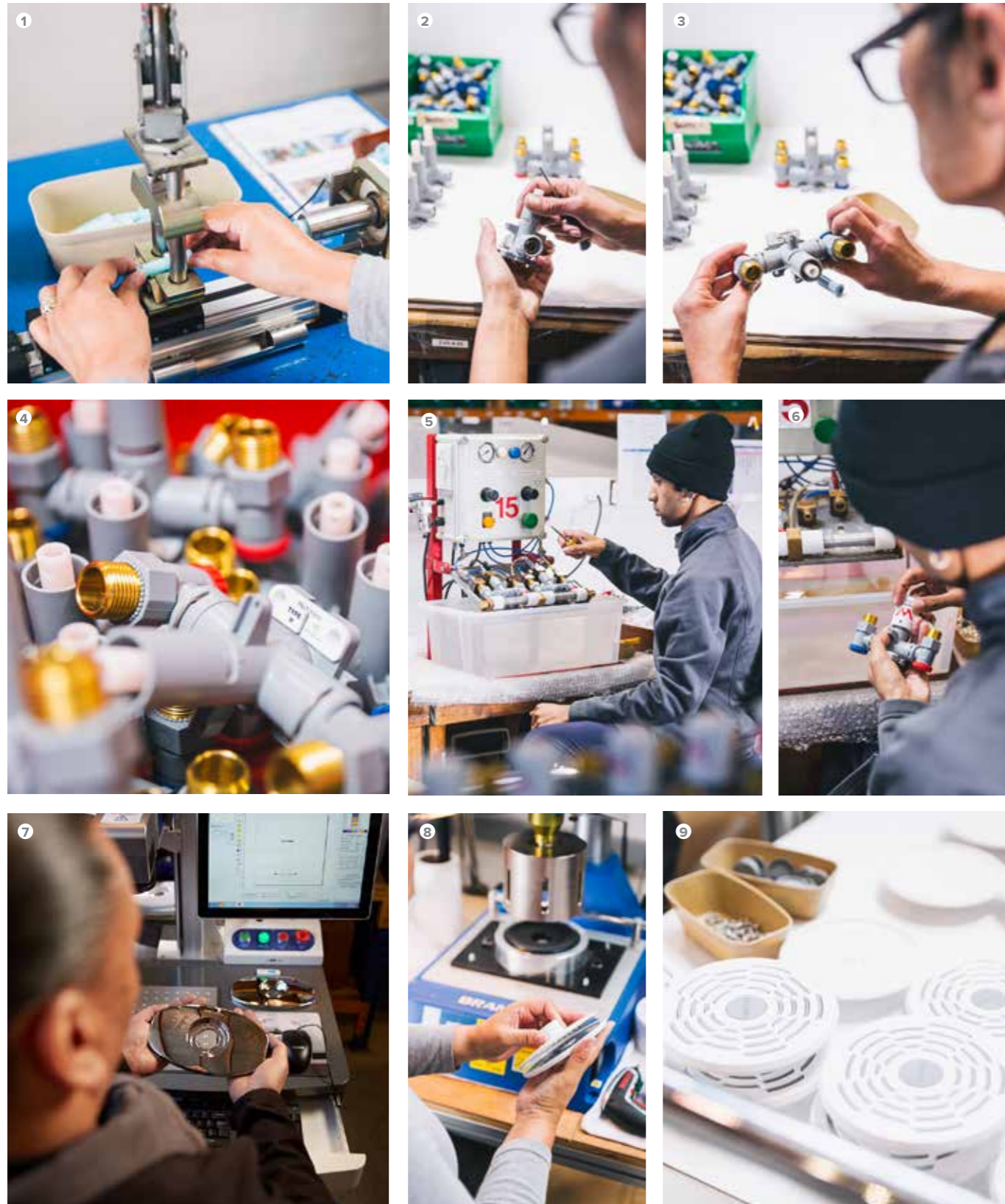
From left to right, top to bottom: 1 Friction welding the rotor • 2 Fixing the rotor into the mixer body • 3 Inspecting an assembled Designer '86 Feltonmix™ Mixing Valve • 4 Pressure testing the mixing valve • 5 Fixing the control sleeve onto the mixing valve • 6 Engraving the Felton logo and the hot/cold indicators onto the Designer faceplate • 7 Assembling components of the Designer III shower rose ready for sonic welding • 8+9 Designer III shower rose fresh out of the sonic welding machine
