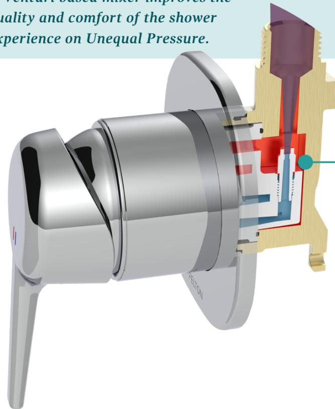
The Venturi works by using the high pressure cold water velocity to draw the low pressure hot water through at an increased rate, providing a balanced shower on unequal pressure.
