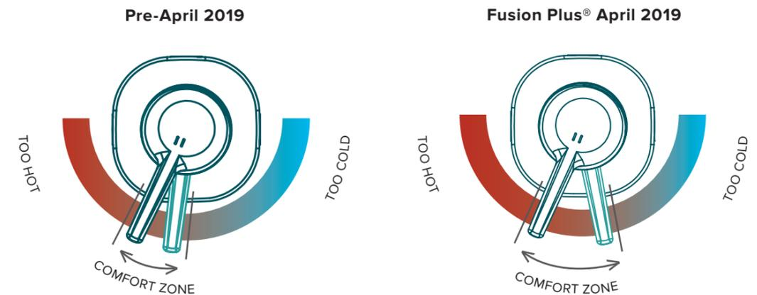
\*Improvement on Unequal Pressure Situations when compared to Felton Fusion™ & Fusion Plus™ shower mixers prior to April 2019
