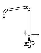
Fit overhead shower arm onto diverter valve and secure grub screw on shower arm into the white bushing
