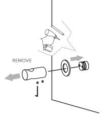
Loosen grub screws from the lower mounting bracket using a 2.5mm allen key and remove the easy fit. Mark and use screws to fasten easy fit into place, then slide chrome flange over.
