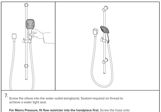
the elbow and handpiece and attach the handpiece to the slider on the rail.
