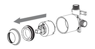
2. Remove the insert disc using long nosed pliers by carefully inserting the nose of the pliers into the indicated areas A & B.
