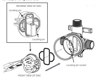
5. Reassemble mixer. Ensure that both black lines marked on the cartridge and cartridge nut are aligned when the mixer is in full cold position as shown in Figure 1.
