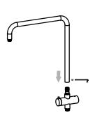
Fit overhead shower arm onto diverter valve and secure grub screw on shower arm into the white bushing 4. using the 2.5mm allen key.
