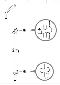
Fit the entire assembly onto wall by tightening the grub screws on the 7. bottom and top mounting bracket using the 2.5mm allen key.
