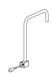
Assemble the top section by aligning the arm with the top mounting bracket. Once aligned tighten the screw to lock 2. the bracket into place.
