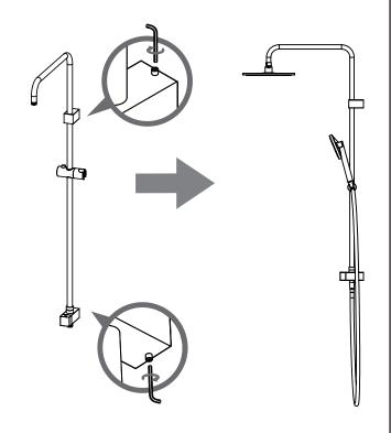
8. Fit the entire assembly onto wall by tightening the grub screws on the bottom and top mounting bracket.
