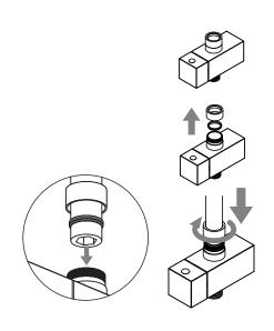
Fit the centre rail to the bottom bracket by un-screwing the thread and inserting the rail into the bottom bracket. Re-assemble the existing layout as shown and tighten to 3. lock into place.
