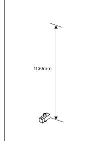
Before fitting, ensure that there is at least 1130mm from the top of the ceiling to the bottom mounting bracket (as this also acts as the 1. plumbing inlet).
