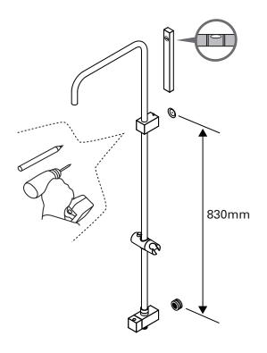
Measure 830mm from centre of the wingback to the centre of the top mounting bracket.
