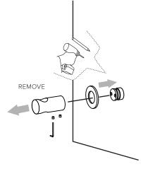
Loosen grub screws from the lower mounting bracket using a 2.5mm allen key and remove the easy fit. Mark and use screws to fasten easy fit into place, then slide chrome flange over.
