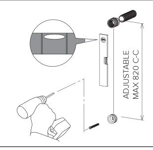
Screw the Top Inlet Mounting Bracket onto the water outlet (wingback & barrel nipple). Sealant is required on thread to achieve a water tight seal. Mount the brackets into the desired position on the wall (adjustable MAX 820mm C-C), ensuring that 2. they are in the correct orientation.
