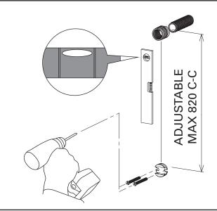
Screw the Top Inlet Mounting Bracket onto the water outlet (wingback & barrel nipple). Sealant is required on thread to achieve a water tight seal. Mount the brackets into the desired position on the wall (adjustable MAX 820mm C-C), ensuring that 2. they are in the correct orientation.
