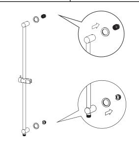
Fit the flanges over both brackets of the rail. Then mount the rail onto the brackets in place. Ensure that both rail and bracket are secured.
