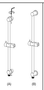
Tighten the grub screws on the rail with an allen key (A). Push the flanges firmly against the wall (B).
