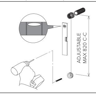
Screw the Top Inlet Mounting Bracket onto the water outlet (wingback & barrel nipple). Sealant is required on thread to achieve a water tight seal. Mount the brackets into the desired position on the wall (adjustable MAX 820mm C-C), ensuring that 2.
