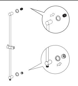
Fit the flanges over both brackets of the rail. Then mount the rail onto the brackets in place. Ensure that both rail and bracket are secured.
