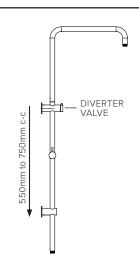
Mark down vertical between 550mm and 750mm from centre of water outlet. Warning: Ensure no water pipe or power cable in wall at this location.
