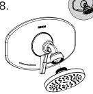
Ensure the rubber seal for shower head is intact then fit and tighten the shower head to the screw cap and stem. Check operation. Handle should swing from right to left from OFF to HOT. Total movement is about 130°.
