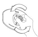
Rotate slotted sleeve on valve body (projecting from central hole of wallplate) anti-clockwise.
