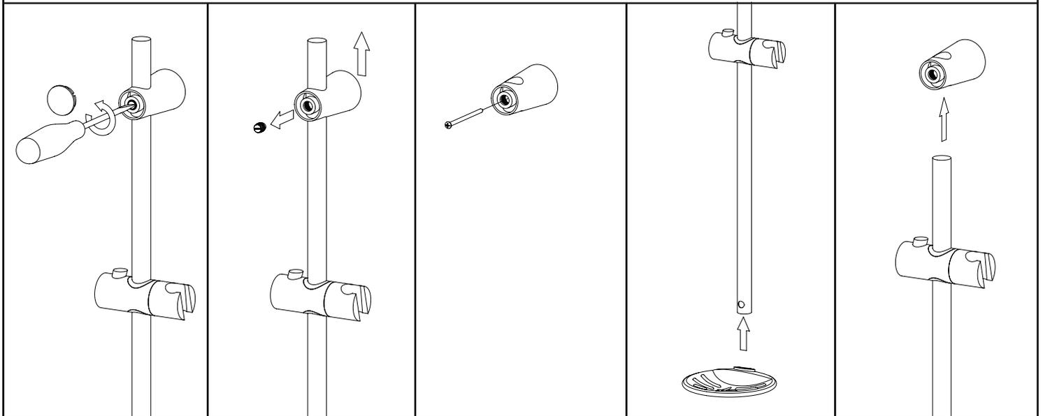
1. Remove the bracket cap and unscrew the plastic tightener.
