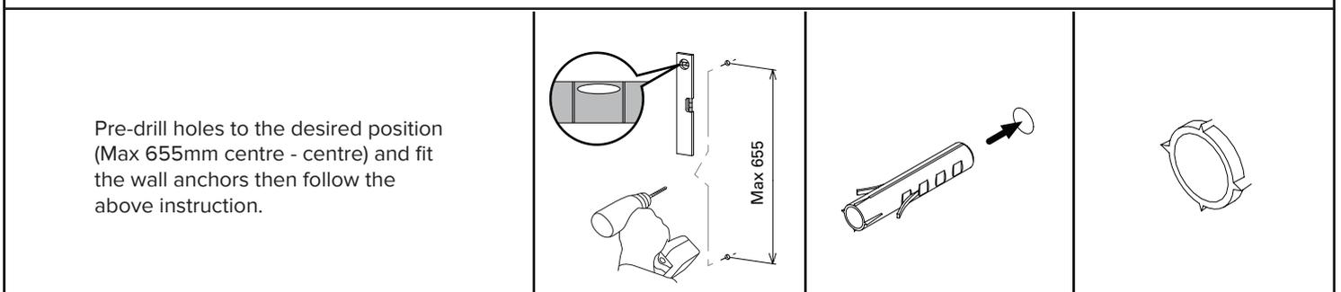
Pre-drill holes to the desired position (Max 655mm centre - centre) and fit the wall anchors then follow the above instruction.
