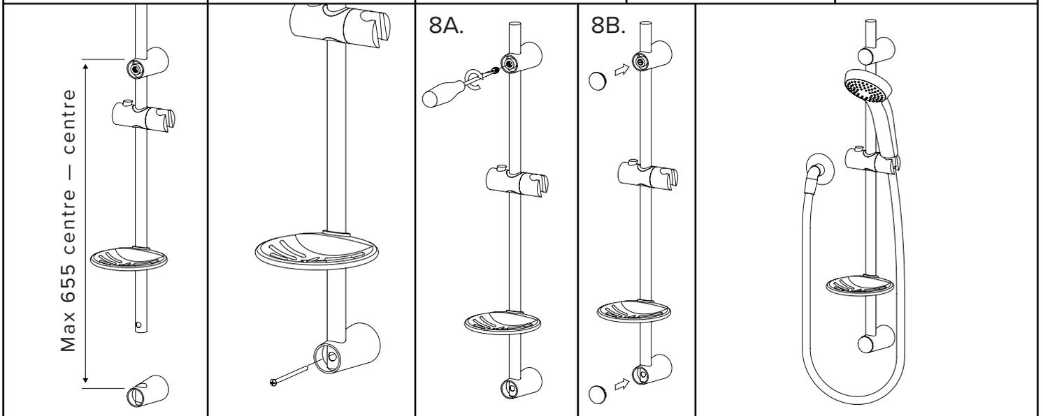
6. Hold the rail and position the bottom bracket into the desired position (max distance 655mm C-C).
