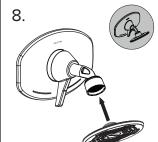
Ensure the rubber seal for shower head is intact then fit and tighten the shower head to the screw cap and stem. Check operation. Handle should swing from right to left from OFF to HOT. Total movement is about 130°.
