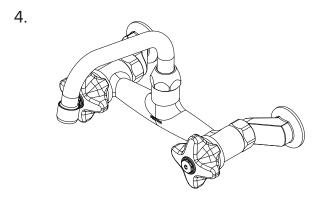
Turn on the water supply and check for leaks.
