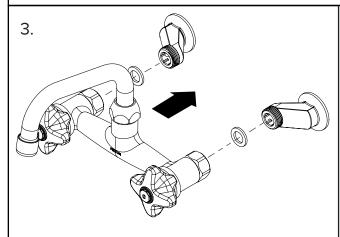
Tighten the nuts at the back of the body onto the offsets ensuring the rubber washers are in place.
