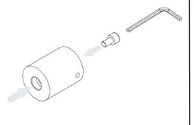
From the supplied pack, loosely fit the brass fitting and hex bolt into the wall mount as shown.
