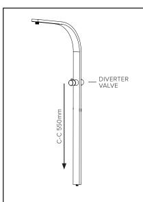
Mark down vertical of 550mm from centre of water outlet to bottom wall fixing position.
