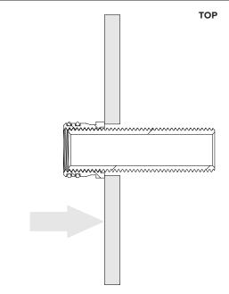
Screw the top easy fit onto water outlet till it is  $\label{eq:3.2} \textbf{3.} \ \ \text{flush against the wall face}.$
