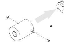
A. With an allen key remove the two grubscrews from the bottom mount to remove the brass wall fitting. Keep these grubscrews as they will be reused when fixing the rail to the wall.
