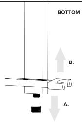
A. Unscrew hose adaptor from bottom of the column.
