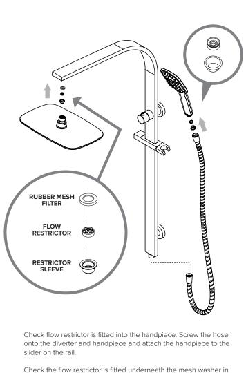
the rain head. Fit the rain head onto the thread on the end of the
