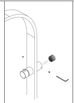
2. Loosen grub screws on body of diverter valve and remove the brass easy fit.
