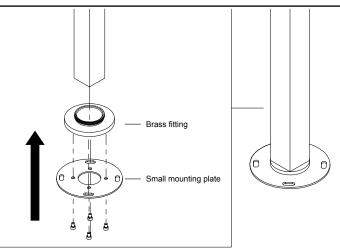
3A. Fix the small mounting plate onto brass fitting from the bottom with screws supplied.
