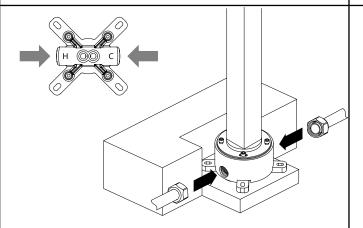
9. Connect the hot and cold water source to the mixer location. Make sure to purge the pipe before connecting to the mixer. Test water tightness.
