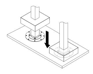
10. Upon completion of floor finish, push the base plate until flush with floor and covering mixer hole. Silicone is optional under the inner edge of the plate.
