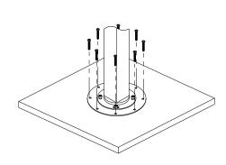
8. Using the 8 supplied wood screws, fix the bath filler into the wood floor
