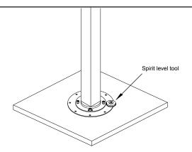
7. Check that the bath filler is level with the supplied spirit level tool.
