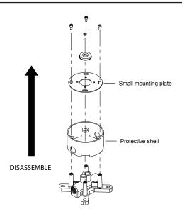
2. Remove screws, small mounting plate, protective shell and spirit level.
