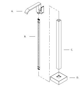
1. Preassemble the above parts in the the same order. Make sure that the tall base plate (D.) is fitted before proceeding.
