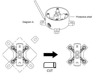
4. Using the protective shell as a template to mark the mixer (See Diagram A). With a hacksaw, cut the floor mounting points of the mixer as marked. This is so the mixer will fit in the ø100mm hole later in the installation.
