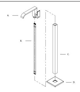
1. Preassemble the above parts in the the same order. Make sure that the short base plate (D.) is fitted before proceeding.
