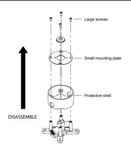
2. Remove screws, small mounting plate, protective shell and spirit level.
