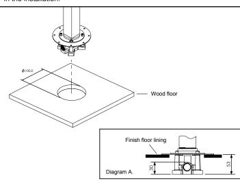
6. Before cutting the hole, ensure that there is sufficient depth below the wood floor for the mixer (See Diagram A). With a hole saw, cut a ø100mm hole in the wood floor. The hole should not exceed 100mm diameter or there will be insufficient surface area for
