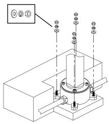
8. Fit the mixer back into position and secure into place with the washer and nut of the Dynabolts.
