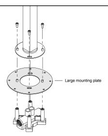
5. Fix the bath filler assembly, large mounting plate and mixer together with the supplied screws. Ensure that the supply pipes are aligned and fitted into the mixer before tightening the screws.
