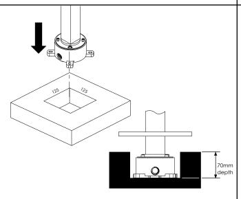
5. Cut a 125 x 125mm hole by 70mm deep into the concrete. Make sure the cut hole provides sufficient space to connect water sources and a level surface for the mixer to be fixed upon. <u>The hole should</u> <u>not exceed 150mm</u> or there will be insufficient surface area for mounting.
