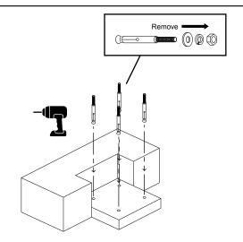
7A. Drill four ø8mm x 45mm deep holes in the marked locations. 7B. Remove the nut and washers from the supplied Dynabolt and fit Dynabolt into each drilled hole.
