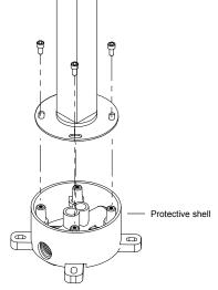
4. Fix the bath filler assembly, protective shell and mixer together with the supplied screws. Ensure that the supply pipes are aligned and fitted into the mixer before tightening the screws.
