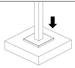
10. Upon completion of floor finish, push the base plate until flush with floor and covering mixer hole. Silicone is optional under the inner edge of the plate.
