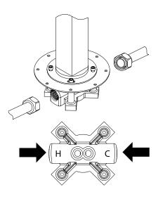
9. Connect the hot and cold water source to the mixer location. Make sure to purge the pipe before connecting to the mixer. Test watertightness.
