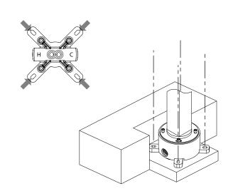
6. With the mixer connect and in the correct position, mark the four floor mounting points of the mixer.
