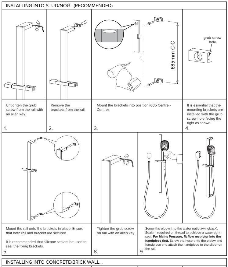
Pre-drill holes to 685 Centre - Centre and fit the wall anchors then follow the above instruction.
